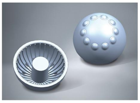
Injection molded globoid-shaped part using additively manufactured mold cores with conformal cooling
